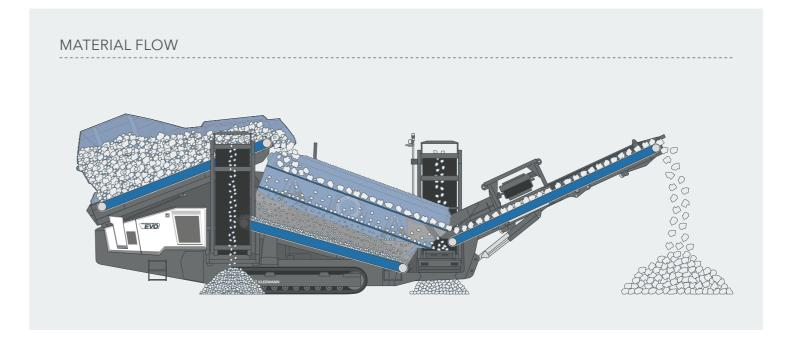
With its proportionally controlled running gear, the plants for coarse screening can be moved quickly and precisely, whether from the low-loader to the application site or within the work site. The side discharge conveyors can be folded without the need to assemble or disassemble any components, thereby reducing set-up times.
