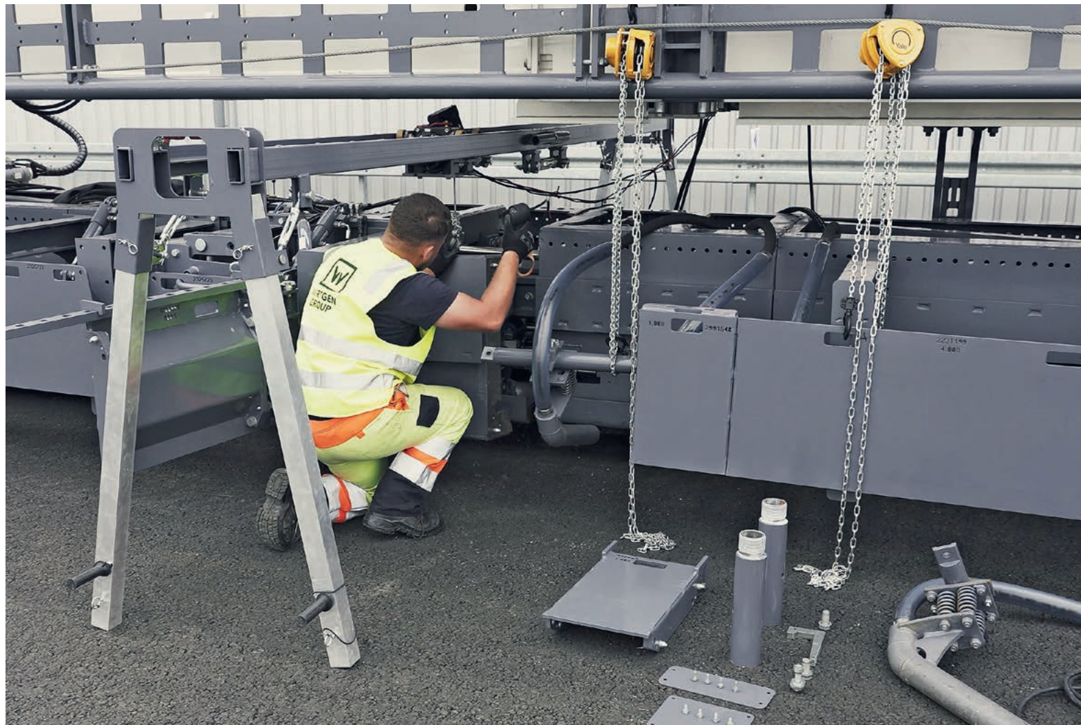
The practical, optionally available lifting device enables even easier removal and installation of extension elements.
