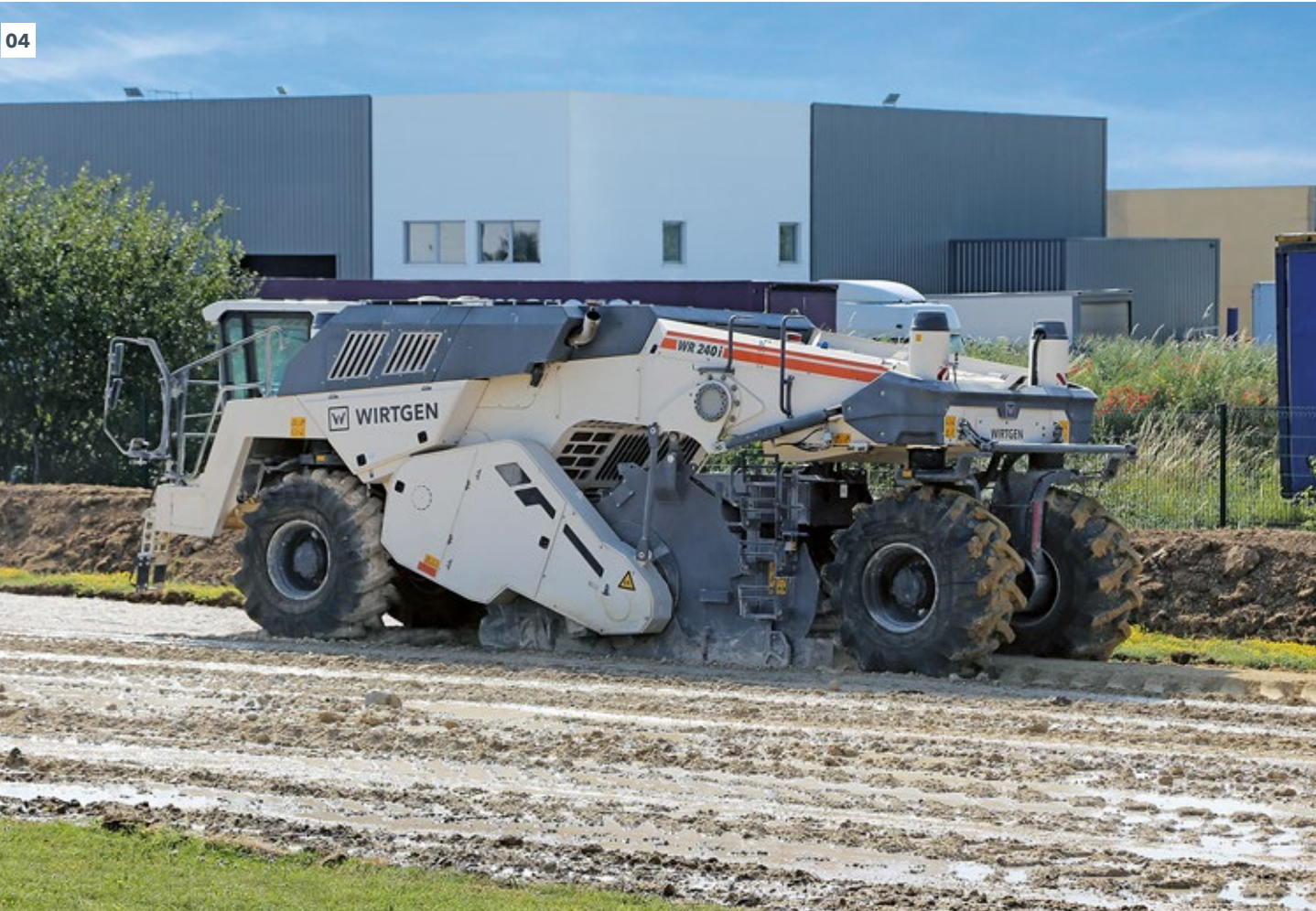
01 - 04 Soil stabilization involves transforming sub-bases with insufficient bearing capacity into soil that is perfect for paving and compaction.
