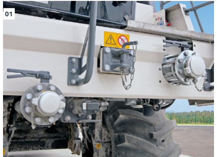
01 The filling connector for foamed bitumen is easily accessible.
