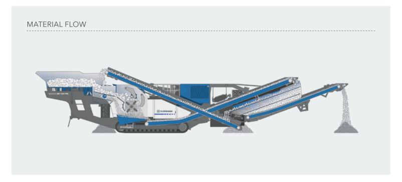
The MOBIREX MR 130i PRO excels with outstanding product quality and very high product output. The Continuous Feed System (CFS) guarantees continuous crusher utilisation. Thanks to the fully hydraulic crusher gap adjustment, machine parameters can be adapted quickly to the application. The overload system ensures effective
