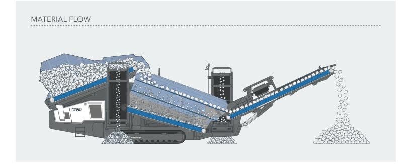
With its proportionally controlled chassis, the coarse screening plant can be moved quickly and precisely, to the application site or within the construction site. The side discharge belts can be folded without the need to assemble or disassemble any components, thereby reducing set-up times. More versatility is achieved thanks
