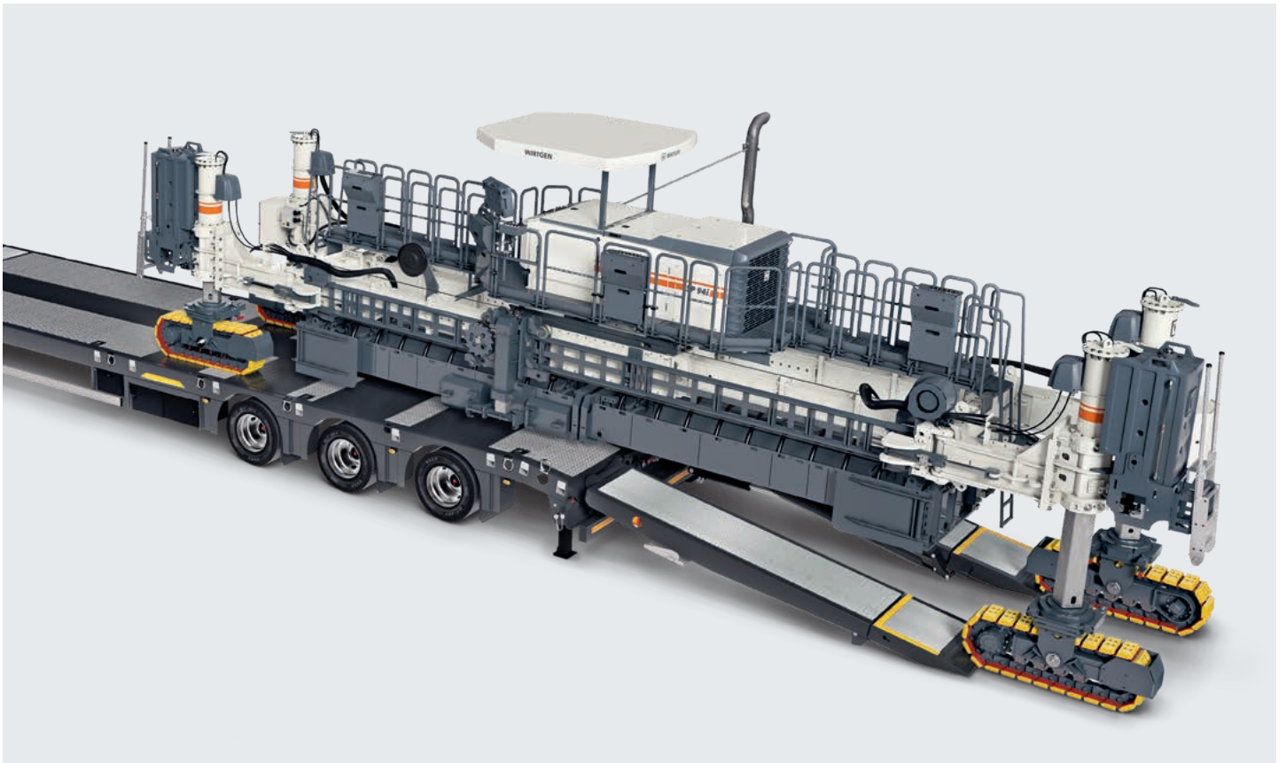
Hydraulic swivel arms for easy transport and a high degree of flexibility on the job site.
