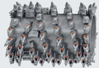
Standard Milling Drum Milling width: 1,300 mm Milling depth: 0 - 330 mm Tool spacing: 15 mm
