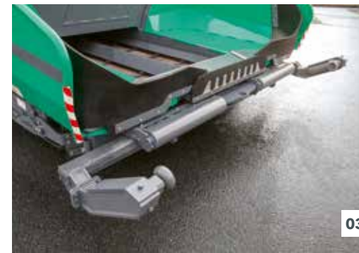
01 Choice of engine speed ranges 02 Steering with preselected steering angle 03 Truck Hitch
