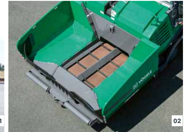
01 Independently operated hopper wings. 02 The large material hopper holds 14.3 tons (13 tonnes).
